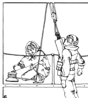
6 HOIST MOB ABOARD
