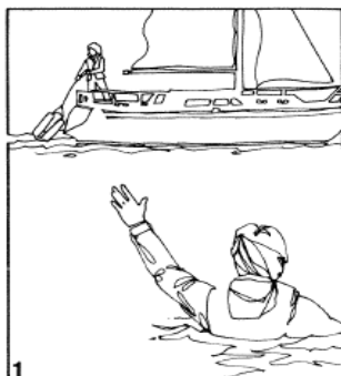
1 STOP THE BOAT IMMEDIATELY near MOB. Sailboats head into wind. Luff all sails. Maintain visual contact with MOB at all times. DEPLOY LIFESLING. Throw off transom of boat. It will trail behind boat to end of floating tether line.
