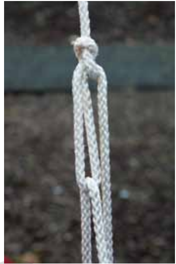
The trucker's hitch does not slip when tied properly.
