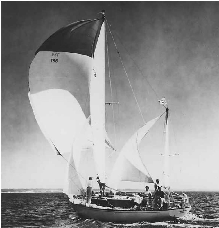
Yawl Carrying Spinnaker and Mizzen Staysail
